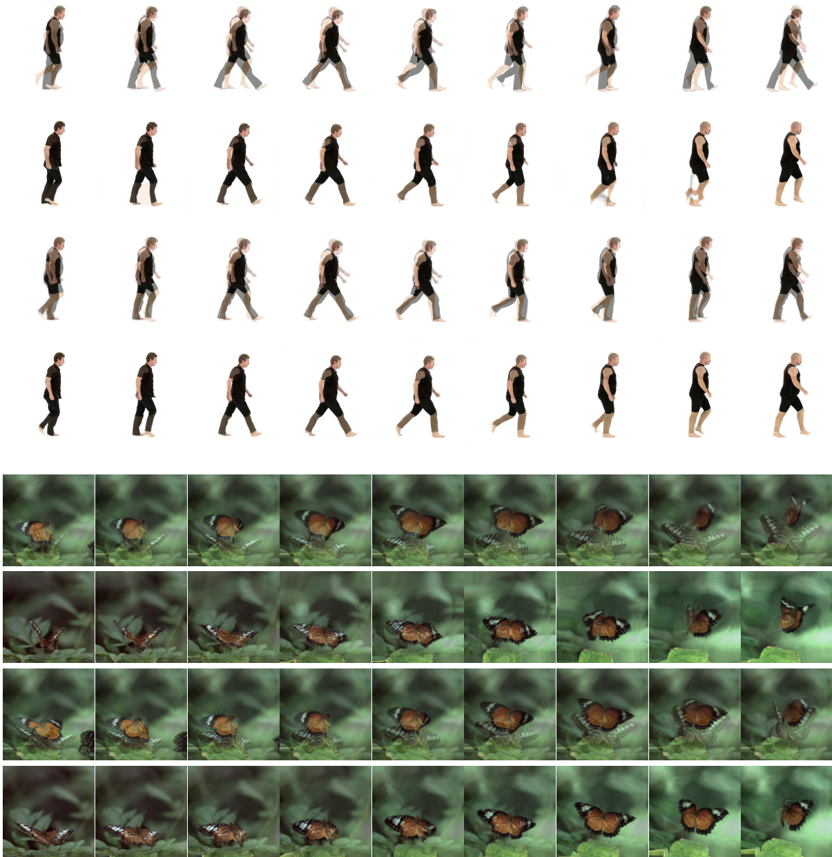
Figure 11: Benefits of temporal synchronization. In each example, the four rows show (1) blending of the input videos, (2) the result of directly performing spatial optimization without synchronization and the resulting artifacts, (3) blending of the temporally synchronized videos, and (4) the final result that combines both temporal synchronization and spatial optimization.
