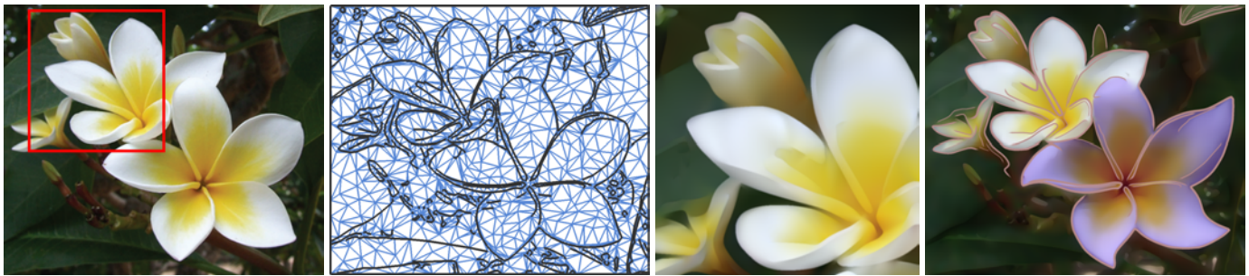
Fig. 1. A raster image converted to a piecewise smooth vector-based representation with curvilinear features. Guided by the feature curves, a multiresolution vector image pyramid enables intuitive editing of the resulting vector graphics. Left: Original image. Middle left: Subdivision surface control mesh for vectorization. Middle right: Magnified (4x) local view of the vectorized image. Right: Combined effects of shape editing, color editing and stylization on the vector representation.
