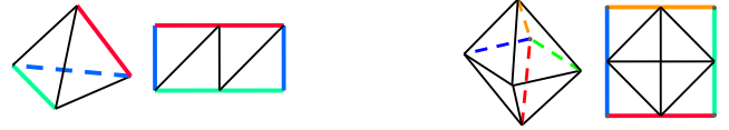
Figure 5: Cutting and unfolding the tetrahedron and octahedron. The colored edges represent the domain cuts.
