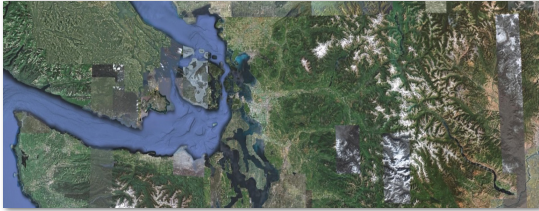
Figure 4: Replacing coarse pyramid levels by downsampling the sparse fine imagery may lead to a patchwork appearance at coarser levels. (Example from Google Earth.)
